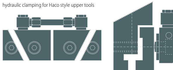
hydraulic clamping for Haco style upper tools
