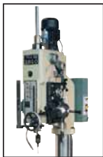
Rosgador husillo patrón Tapping system by lead screw Filetage par vis mere Leistspindel gewindeschneidesystem
